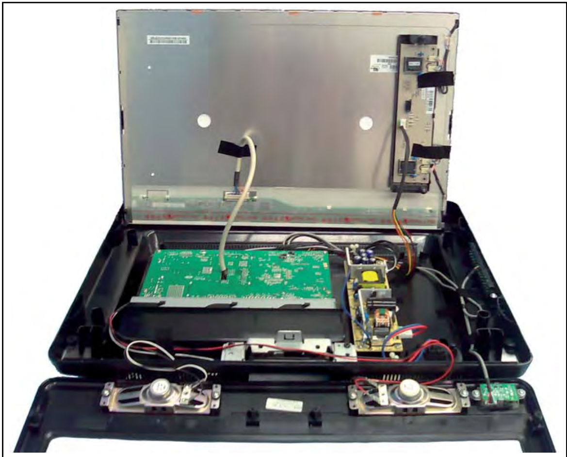
Figure 4-1 Cable dressing (20" model)
